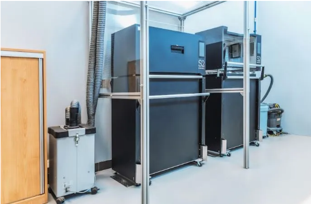
The Sintratec SLS 3D printer used by Johnson Matthey
